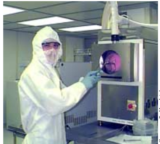
Eddie Bauer (ECpE, UVA) places a silicon wafer in a diffusion furnace.
