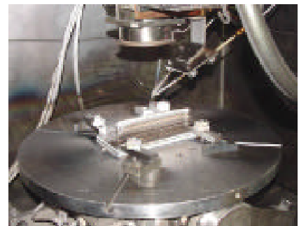
Electron beam welder in the process of freeform fabrication.
