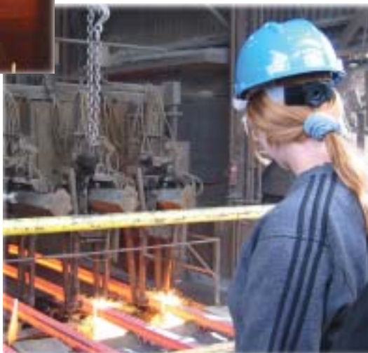
Continuous-cast billets move down the line (Roanoke Electric Steel)
