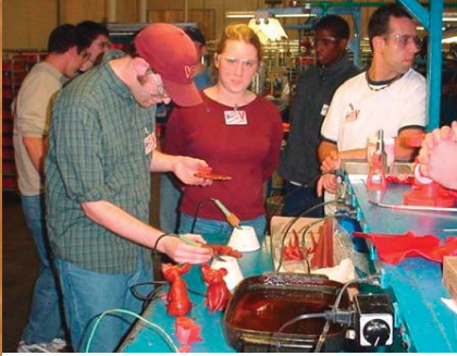
Chris Kessler mounts wax parts onto a tree as part of the investment casting process. This was part of a foundry tour hosted by Conbraco.
