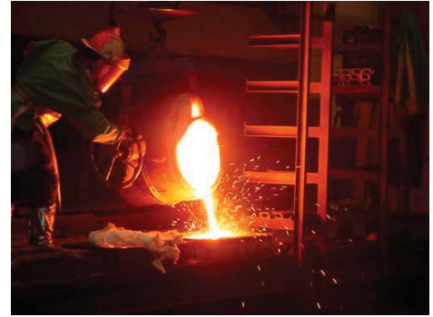
Molten stainless steel is poured into the top of an investment casting. Students watched this as part of a foundry tour hosted by Conbraco.
