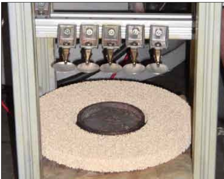
Figure 3. Geometry of the collection substrates attached to the exoskeleton
