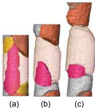
Figure 2. Nanowires after (a) 0, (b) 90 and (c) 270 ps tensile deformation for a strain rate of 1.33 \times 10^9 \text{ s}^{-1} .
