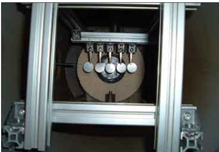
Figure 4. Exoskeleton inside of the vacuum chamber
