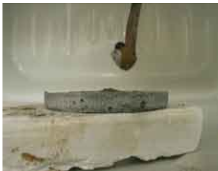
Figure 4. Regolith glass on tip of thermocouple
