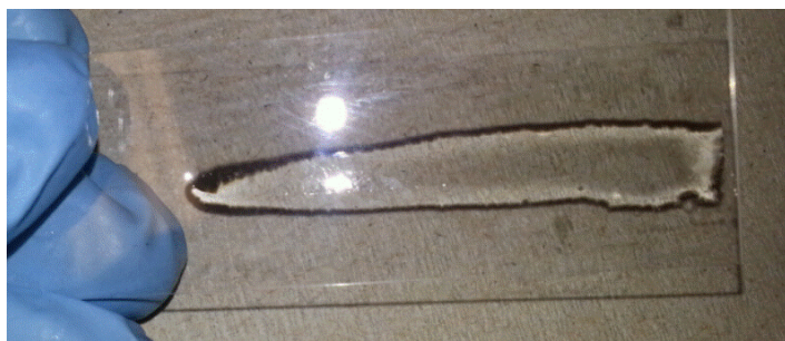
Figure 1: Shape memory polymer fabrication. (a) The polymer casted on glass slide. Note the red dash line indicates the shape of Teflon spacer. (b) Polymer after curing and post-curing.
