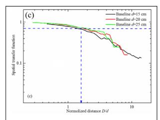
Figure: Gradiometer response curve as a function of distance between ME gradiometer and magnetic source normalized to baseline.
