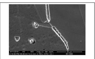
SEM Image of a twin boundary inhibiting intergranular corrosion where it meets a regular grain boundary.
