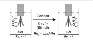
Figure: Schematic depicting the sensor-based sol-gel rheological characterization study and associated measurement principle (i.e., real-time monitoring of gelation processes via sensor signal tracking).
