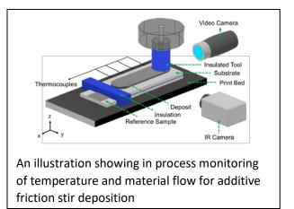
deformation flow, with a comparison between Cu and an Al-Mg-Si alloy. By analyzing the thermal characteristics under a range of processing conditions, we have found generic trends of peak temperature  $T_{peak}$ , exposure time, and cooling rate with respect to the key processing parameters such as tool rotation rate  $\boldsymbol{\Omega}$  and in-plane velocity  $\boldsymbol{V}$  in both materials.
