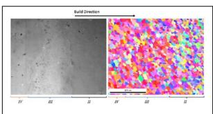
Figure 1: SEM and EBSD images of interface between AA 6022 substrate and AA 6061 deposit. Some differences in texture can be seen across the interface, but otherwise the interface is continuous and free of discernable voids.
