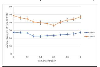
The average number of total defects after primary damage in Ni-Fe concentrated alloys as a function of Fe concentration.
